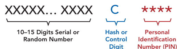
FIGURE 11: Structure for an Uncoded UIN Showing the Identifying Digits, the Hash Control, and the Optional Security Pin
