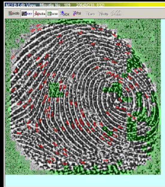
This is a feature extracted image and this shows 109 minutiae detected. This can apparently be matched by existing matching algorithm.
